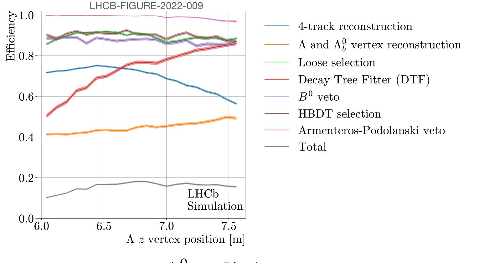
$\Lambda_h^0 \to J/\psi \Lambda$  signal Efficiencies calculated wrt to reconstructible particles (i.e. within acceptance) Low vertex reconstruction efficiency  $\rightarrow$  investigating remedies
