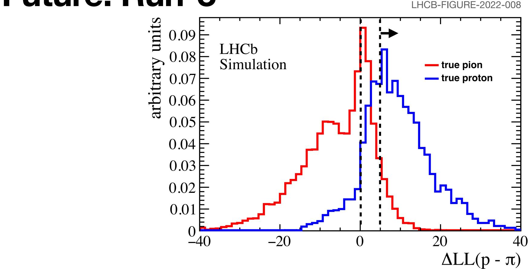
(Very preliminary) The difference in log likelihood between the proton and pion hypotheses for true proton and true pion T tracks with associated RICH2 info in Run 3 MC. RICH2 info was not added to T tracks in Run-2.
