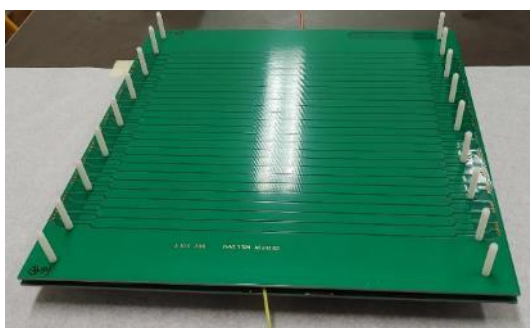
6) assemble the 2nd PCB
