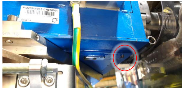
Water leak on BI4.BSW1L1
