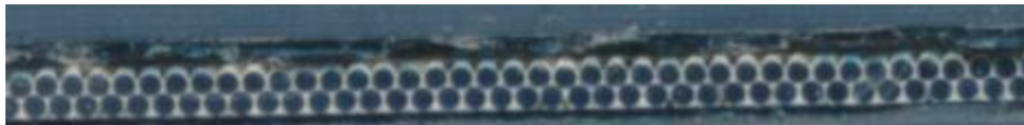
2-layer fiber with glue between fiber and black Kapton foil on the front and back, fixed by epotek glue.
