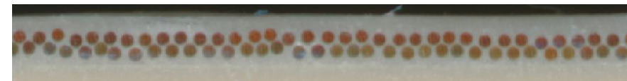
The first 2-layer glueless fiber, in order to keep the material budget to the requirements, fixed by araldite glue.
