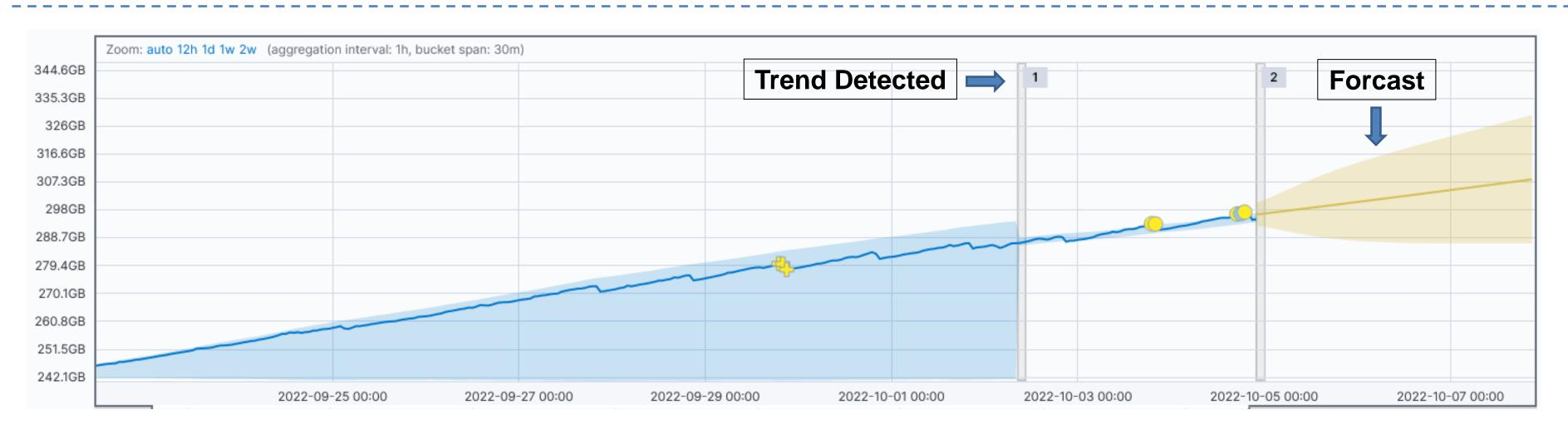
• Total disk usage for a data storage cluster, the yellow portion showing a forecast of the potential usage • The "1" marker is when ELK has detected a trend and sent an alert.
