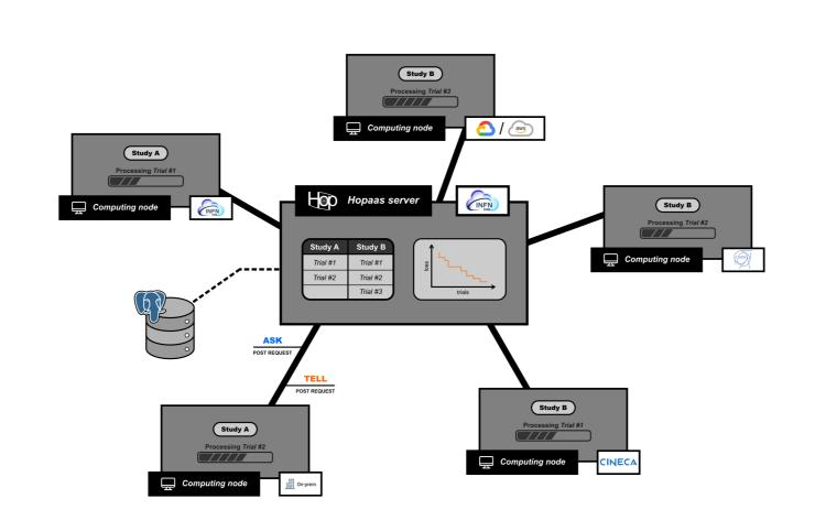
Schematic representation of the Hopaas server as an orchestrator of two optimization studies ("Study A" and "Study B") distributed across five computing instances, and powered by a PostgreSQL database.
