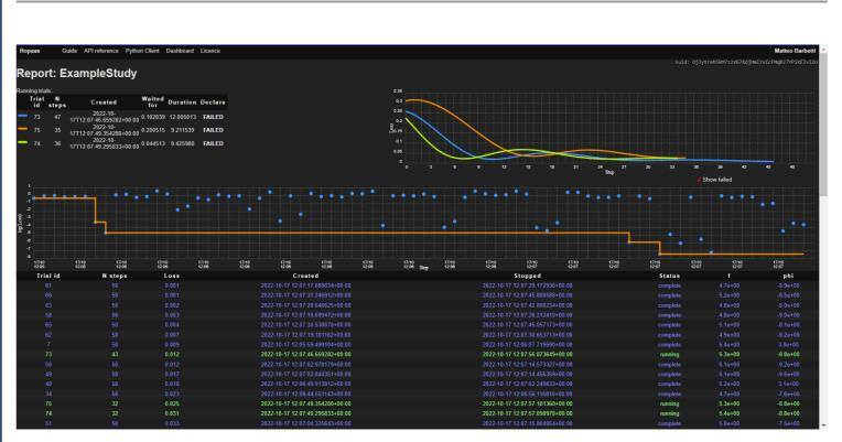
Web dashboard produced by Hopaas for <u>l.infn.it/hopaascolab</u>. The top right plot shows three ongoing trial trainings, while the center plot reports the global status of the optimization study. Finally, the bottom table traces general information from all the trials.
