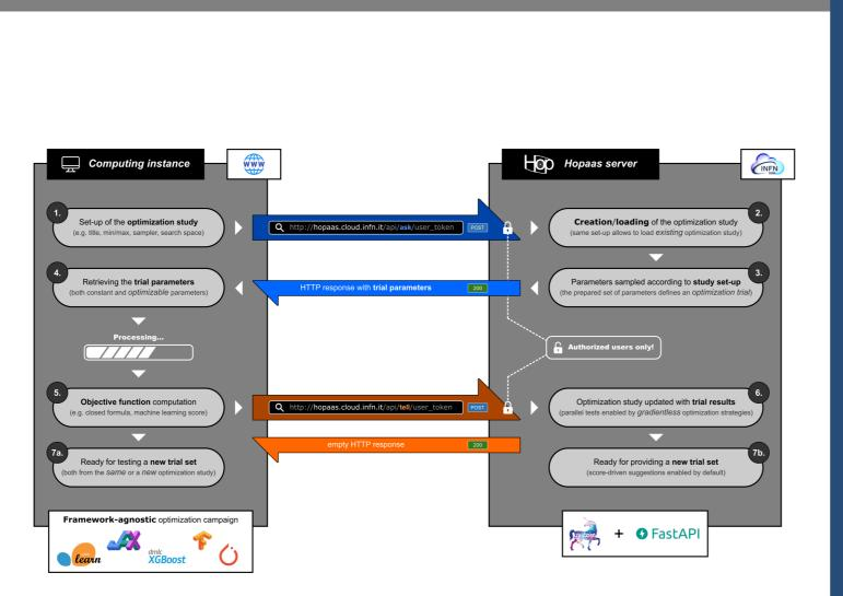
Workflow of the client-server system defined by Hopaas to run optimization studies, and based on an *ask-and-tell* interface where the trial parameters and the objective score computed are retrieved from HTTP requests.
