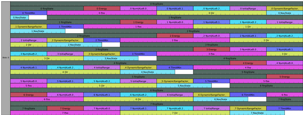
Figure 3: AdePT’s default track layout, visualized by LLAMA. Memory is laid out left-to-right and wraps after 64 bytes. The boxes are colored by LLAMA field and labeled by array index and field name.
