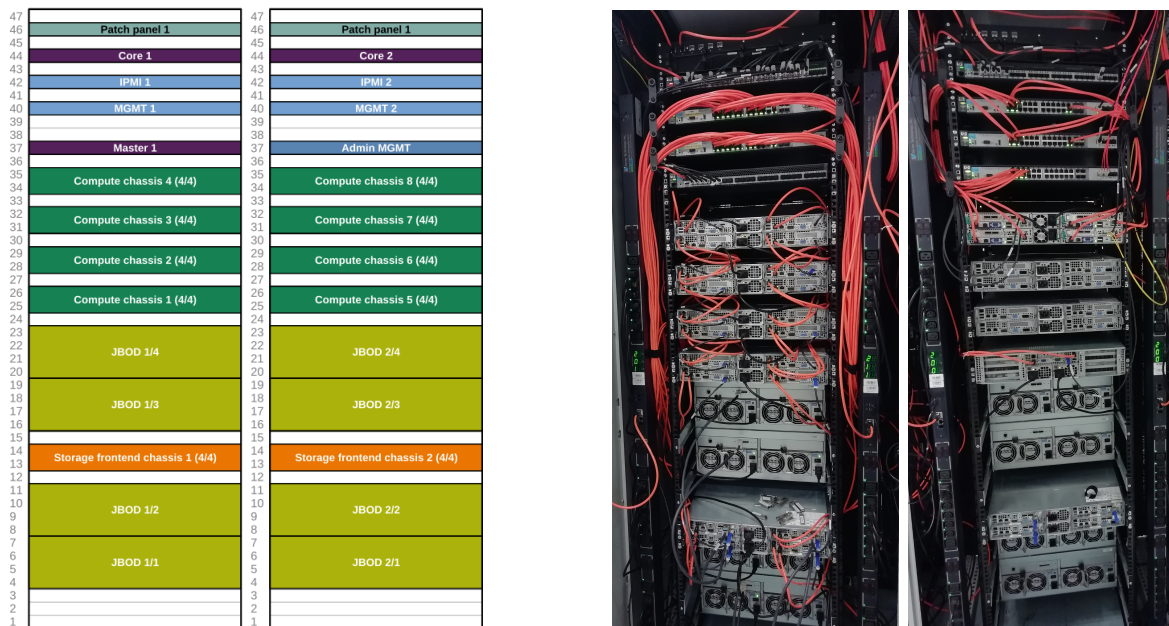
Figure 1. The structure of the a single cell in the Wigner Analysis Facility.
