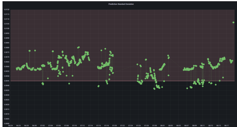
Figure 5. A plot of prediction standard deviation versus time for the CPP program (about two months). A point in the top red shaded area indicates a point outside of the confidence threshold surface which caused the UQ correction protocol to be invoked.
