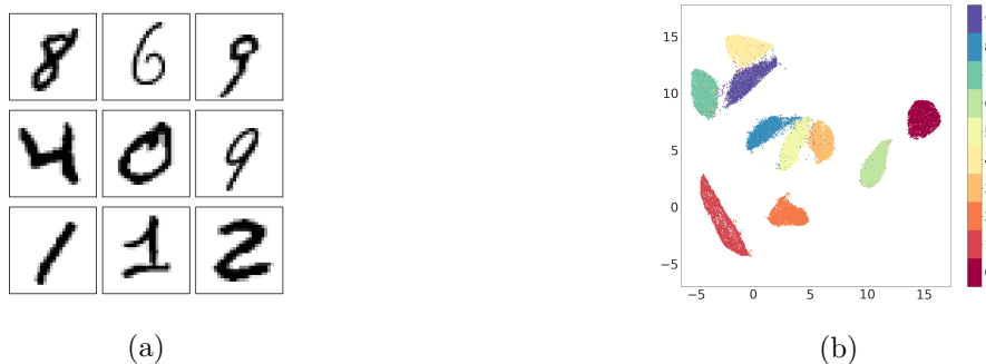
Figure 2: Visualization of the MNIST handwritten digits dataset [4]: (a) Example digits with 784 pixels per images (b) Two-dimensional UMAP representation of the MNIST handwritten digits dataset. Each point represents the image of a handwritten digit. All points are colored according to the digit they represent.
