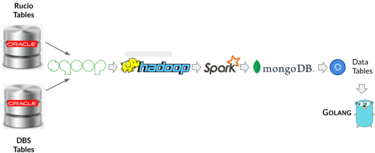
Figure 3. The data pipeline for data management monitoring based on Sqoop dumps of the Rucio and DBS database tables. The monitoring metrics are aggregated with Spark jobs and stored in MongoDB. Metrics are visualised using a web service written in GoLang and based on DataTables [22]
