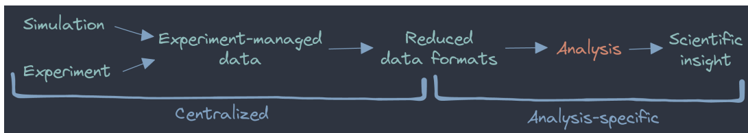
Figure 1. A schematic representation of a typical analysis pipeline. The first half usually corresponds to centralized data processing, while the second half features more freedom and variety of implementations on the part of the single analysis group or even a single analyst.
