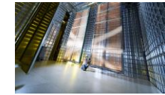
ProtoDUNE: three hundred cubic metre volume prototype Liquid Argon Neutron Detector being constructed at CERN. (© CERN)
