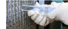
Insertion of lead-fungate crystals (over three times the density of conventional glasses) into the high granularity electromagnetic calorimeter of the ALICE detector giving percent scale energy measurements. (© CERN)
