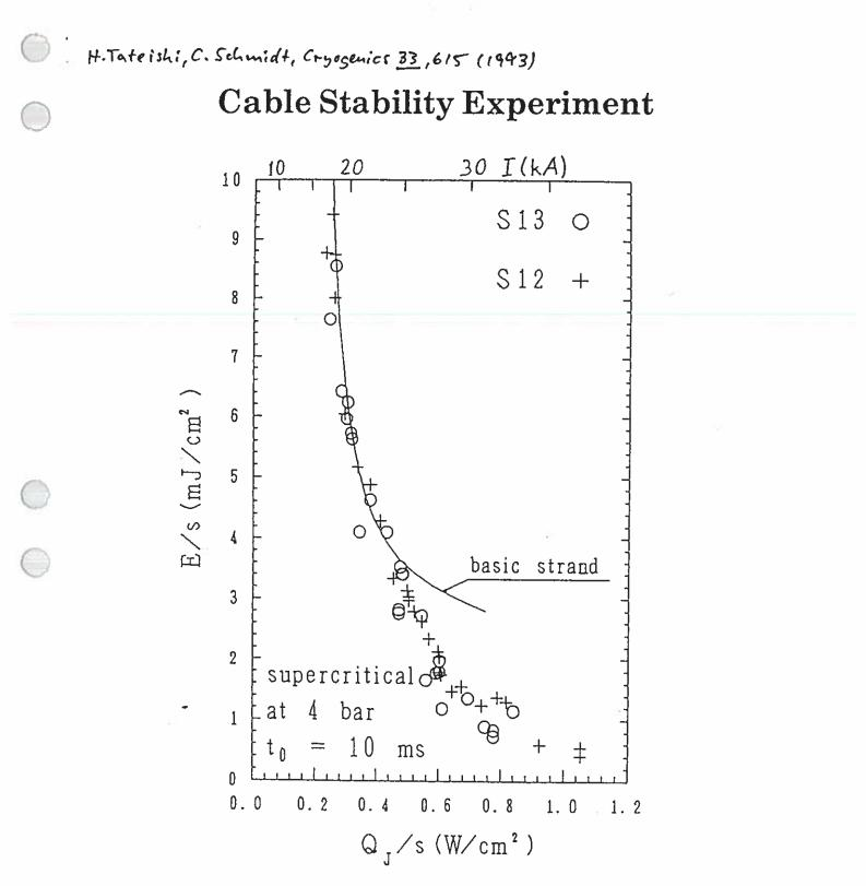
Stability limit in a half cycle sinusoidal external magnetic field pulse of 10 ms duration.
