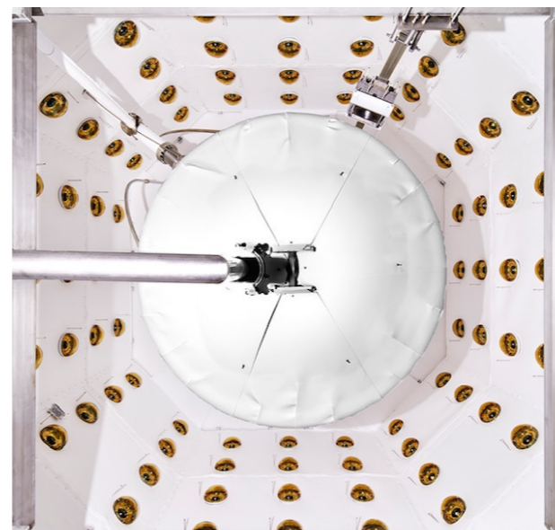
Neutron veto (120 PMTs, Gd-doped water)
