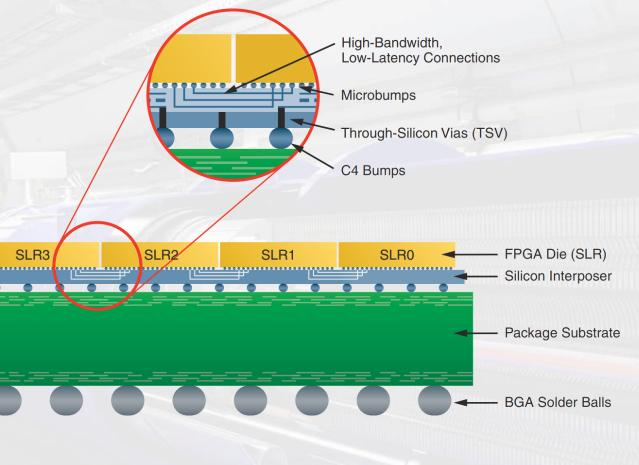
Fig 3: Xilinx FPGA Enabled by SSI Technology\*
