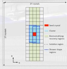
Fig: e/gamma cluster making in RCT algorithm
