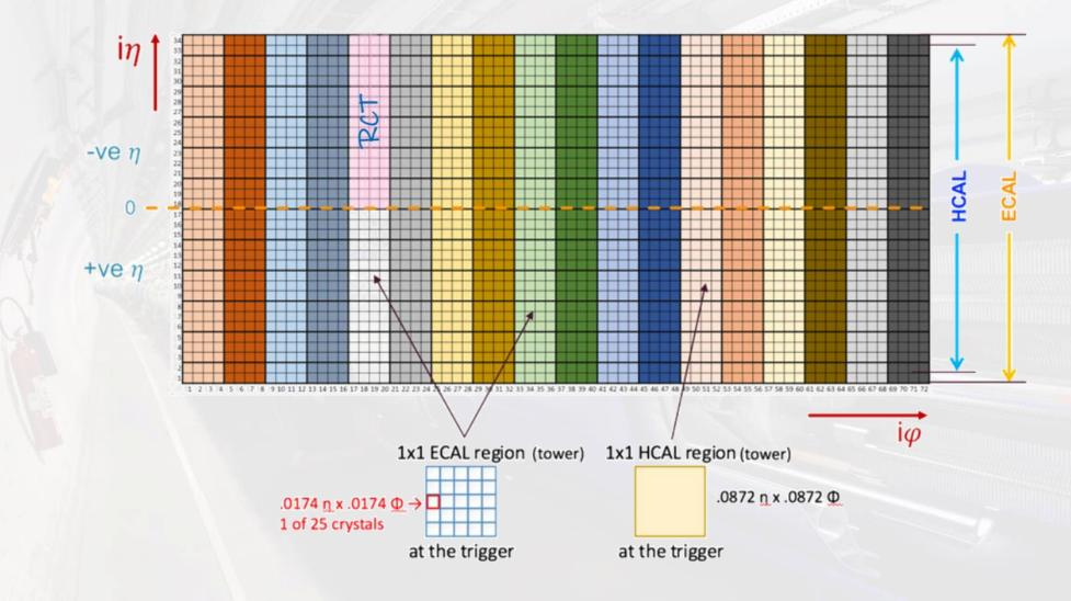
Fig: Barrel calorimeter segmentation
