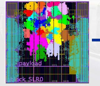
Fig: 39 algorithm placed in 1 SLR (total 117 algorithms for 3 SLR)
