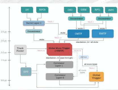
Fig: Muon trigger architecture
