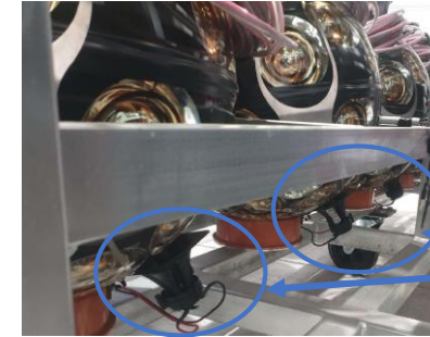
emitters are located at about 10 cm from the DOM south pole
