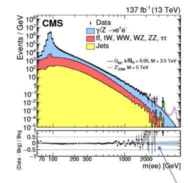
Good agreement up to 1.5TeV Some deviations at high masses point to an excess of electrons w.r.t. muons (stat limited)
