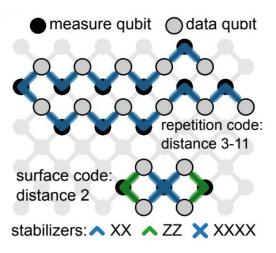
Layout of distance-11 repetition code and distance-2 surface code in the Sycamore processor.
