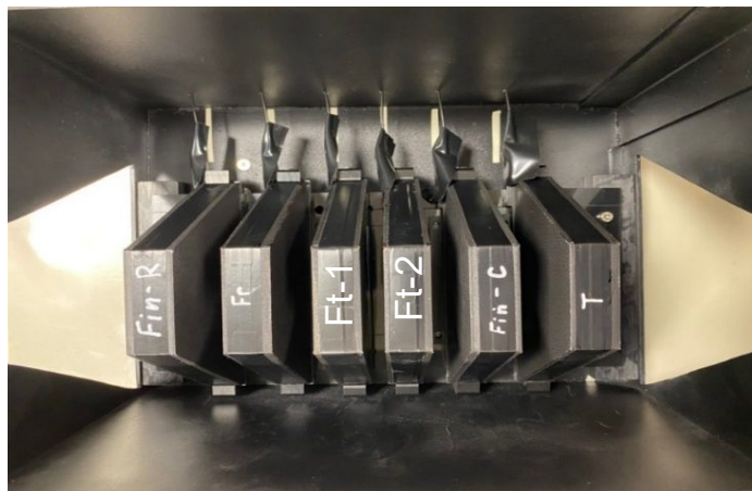
Six different type of tiles assembled for a test beam
