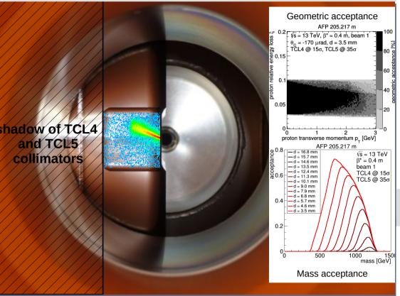
Geometric acceptance: ratio of number of protons of a given relative energy loss ( $\xi=1-E_{proton}/E_{beam}$ ) and transverse momentum that reached the AFP detector to the total number of scattered protons having such ξ and momentum,
