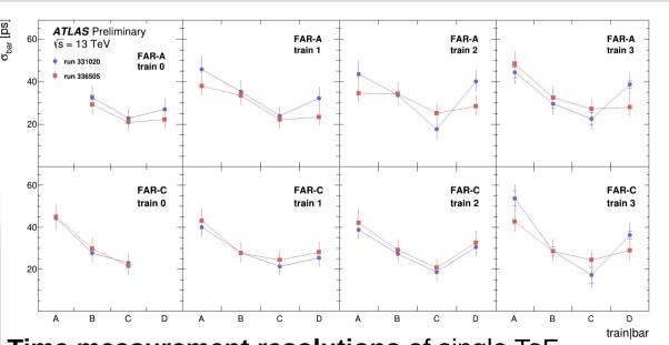
Time measurement resolutions of single ToF channels extracted from AFP calibration data. The time resolutions are extracted from the widths of the distributions of time differences within a single train, between different channels.
