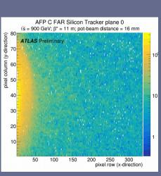
Signal registered in AFP (C Far, layer 0) during pilot beam collisions. Data was taken at injection energy 900 GeV with  $\beta^* = 11 \text{ m optics (no crossing)}$ angle). Stations were outside shadow of TCL4 and TCL5 collimators and beam aperture. Hits in rows 0-50 are mainly from diffractive protons whereas rest of the pattern is most probably due to showers. White areas are due to pixels masked in readout.
