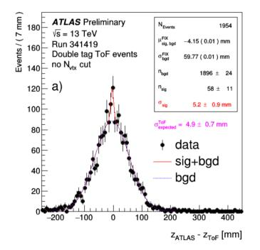
The distributions of z<sub>ATLAS</sub> - z<sub>TOF</sub> measured in events with ToF signals on both sides of the interaction region and primary vertex reconstructed by ATLAS.
