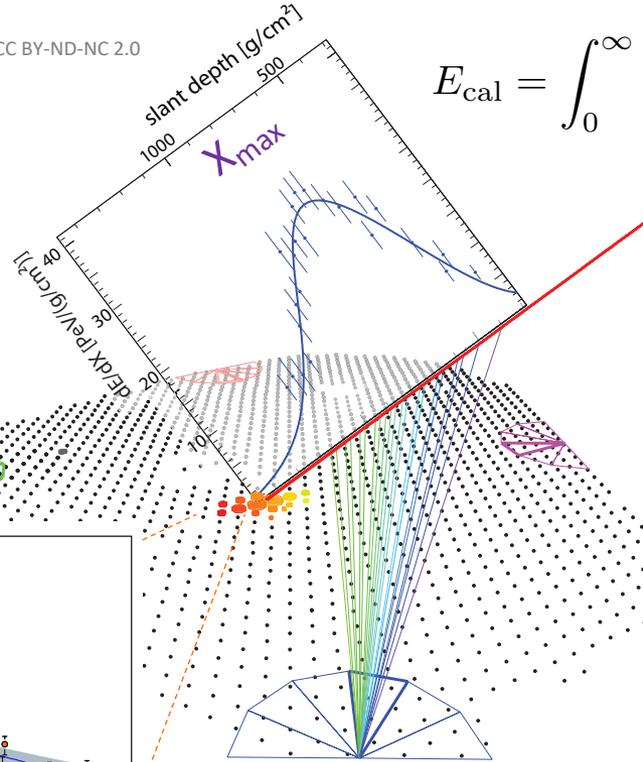
$$E_{\text{cal}} = \int_0^{\infty} \left( \frac{dE}{dX} \right)_{\text{ionization}} dX$$
