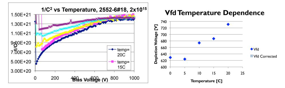
The slope between 5 and 10 °C (largest temperature dependence) has a slope of 7 V,  $= \pm 2\%$  conservatively
