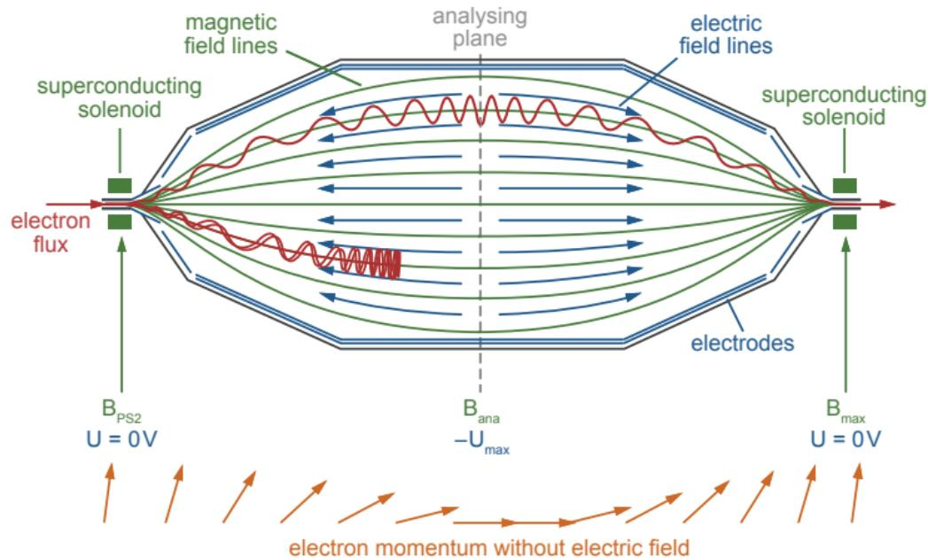
Voltage set points are scanned through to obtain an *integrated spectrum*
