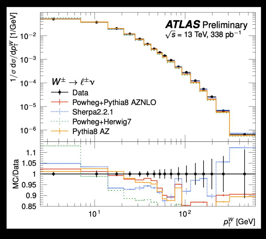
Determine the W boson mass from the dependence of the leptonic transverse momentum ( $p_T$ ) and the transverse mass ( $m_T$ )
