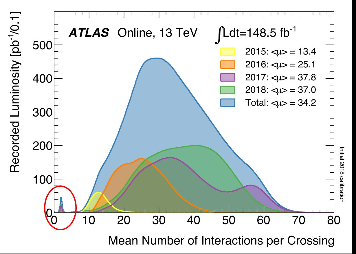
Pile-up events add energy to the recoil and hinder the experimental extraction of W pT
