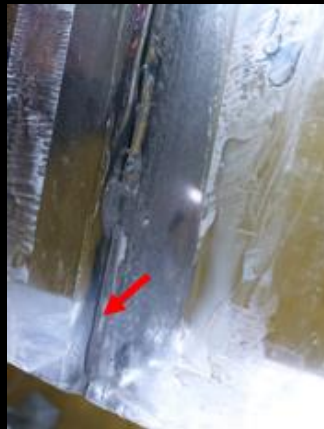
Cracking during annealing
