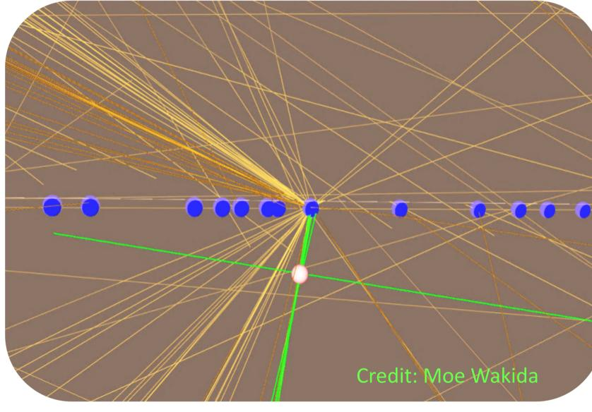
This ATLAS Detector event display shows a number of primary vertices along the proton-proton interaction point (blue) and a displaced vertex emanating from a long-lived particle (pink).
