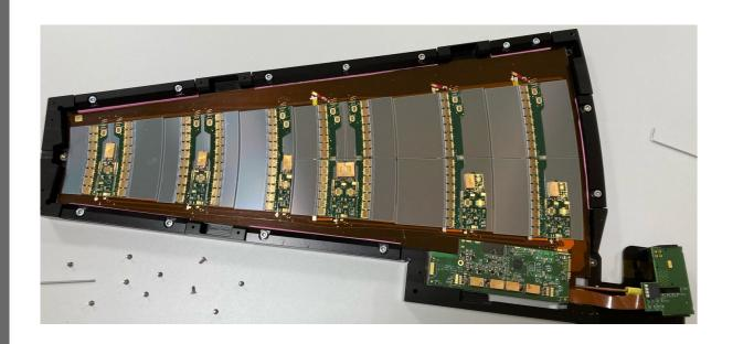
First staves and petals are being populated with the built modules, and tested to check the performance
