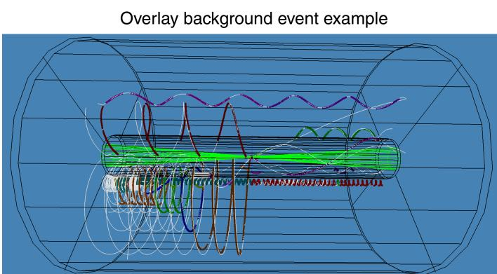
Standard selection: only decays in the **TPC volume** considered; cuts based on track curvature, length, opening angle, and first hit distance to vtx
