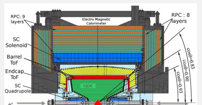
Beam energy: 1.0-2.47 GeV Luminosity:  $1 \times 10^{33} \text{ cm}^{-2} \text{s}^{-1}$  at  $\psi(3770)$  peak
