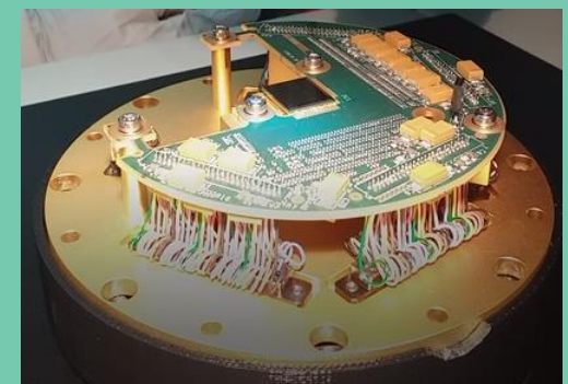
Chip mounted on test assembly
