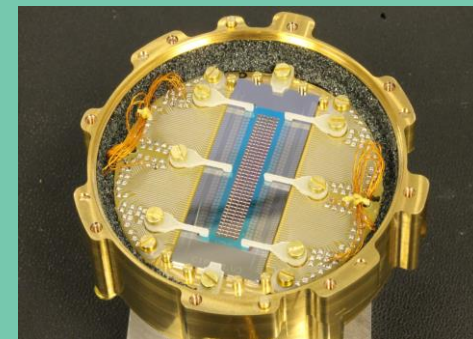
Mounted detector array
