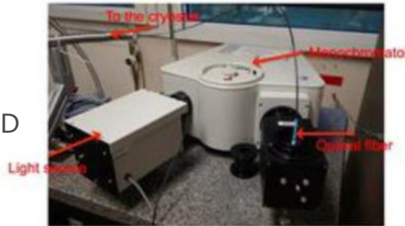
Cryogenic QE test setup
