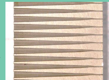
Detailed view of lightpipe structure
