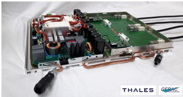
2 kW RF module composed of 50 VDC power supply Cold plate RF board with 2 transistors Output relays
