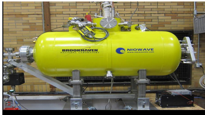
Harmonic cavity in horizontal cold test
