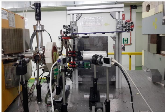
Mixed-field testing with 200 MeV electrons on target, at the CLEAR facility at CERN
