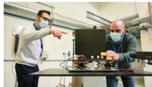
Calibration tests of the Lumina dosimeter in the irradiation facilities at CERN. (Image: CERN)
