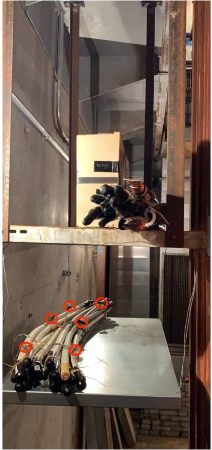
RPLs for MGy cable irradiation
