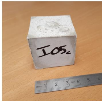
Magnet spacers (grout)
