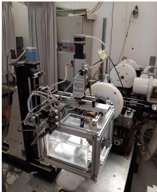
Fiber-based dosimeter testing at TRIUMF (Courtesy of TRIUMF)
