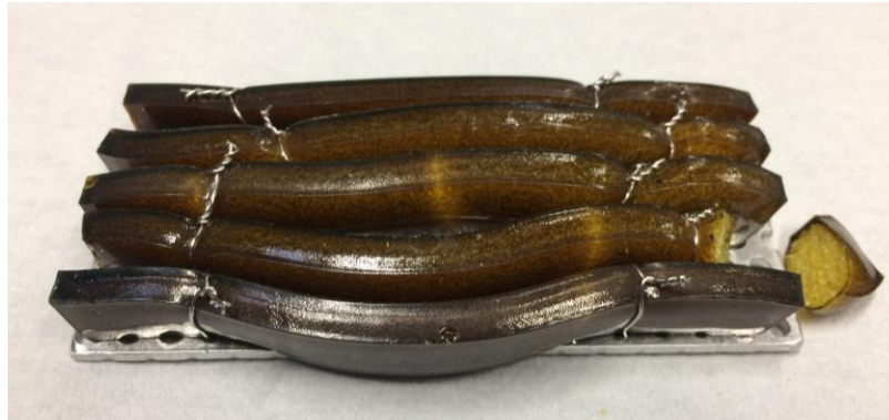
Protective covers for magnets 10 MGy, used in CERN complex Courtesy of C.L. Marraco Borderas (TE-MS)
