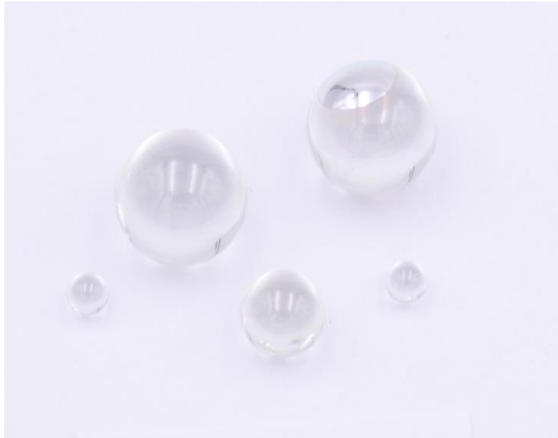
Glass balls, precision components HL-LHC alignment system Non-irr vs 5 MGy Courtesy of M. Sosin (EN-SMM)
