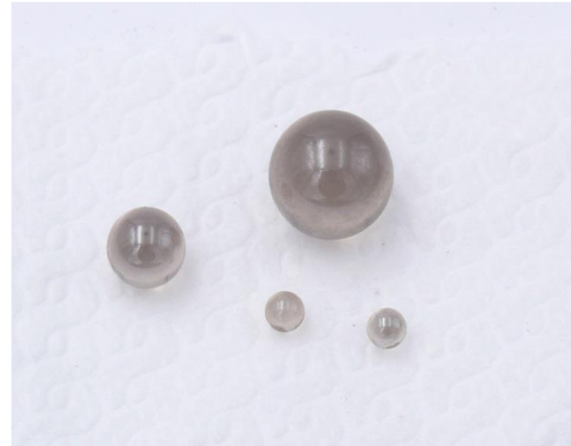
Glass balls, precision components HL-LHC alignment system Non-irr vs 5 MGy Courtesy of M. Sosin (EN-SMM)
