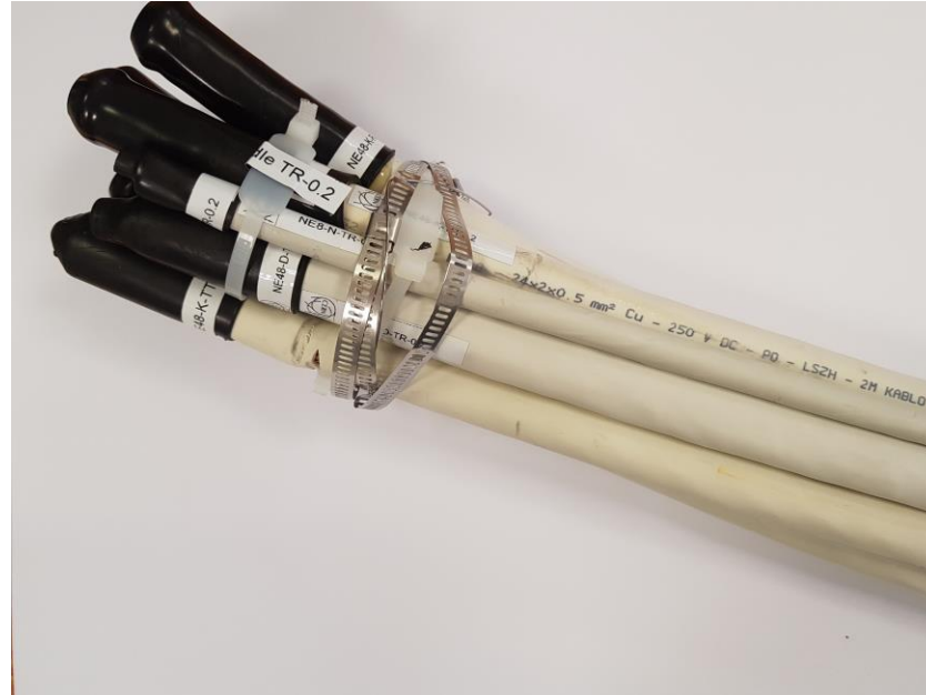
RPL dosimeters attached to irradiated samples
