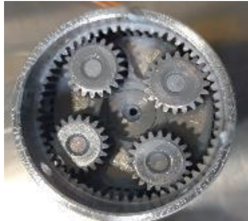
Lubricated motor and gearbox Atlas 0.5 MGy and 3.0 MGy Courtesy V.Rieker, P.Gebolis (TE-VSC)
