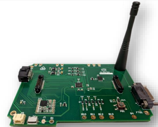
“IoT BatMon: Wireless radiation monitoring at CERN”
