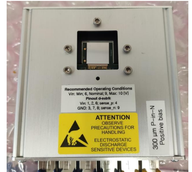
300 \mu\text{m} P-on-N Timepix3 module as a part of the BGI Pixel setup
