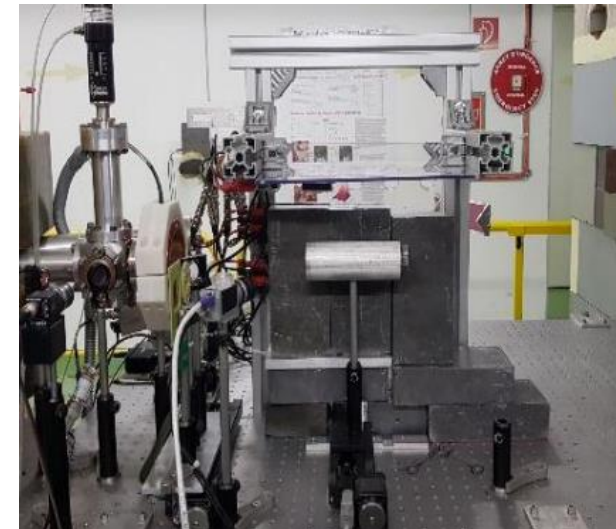
RUN 3 Target with R=2.5cm, Pb shielding in front of side panel Goal: check impact of the shielding on TID and SEU rate
