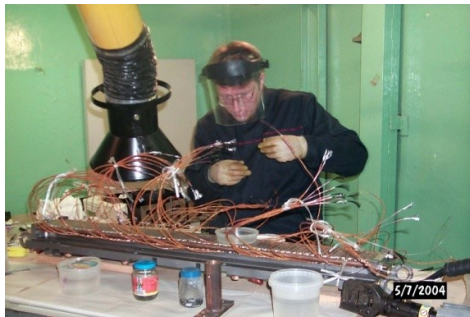
Coils connection by cold welding method
