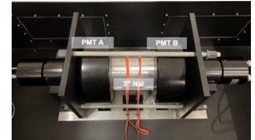
Set-up to reproduce Saint-Gobain observations
