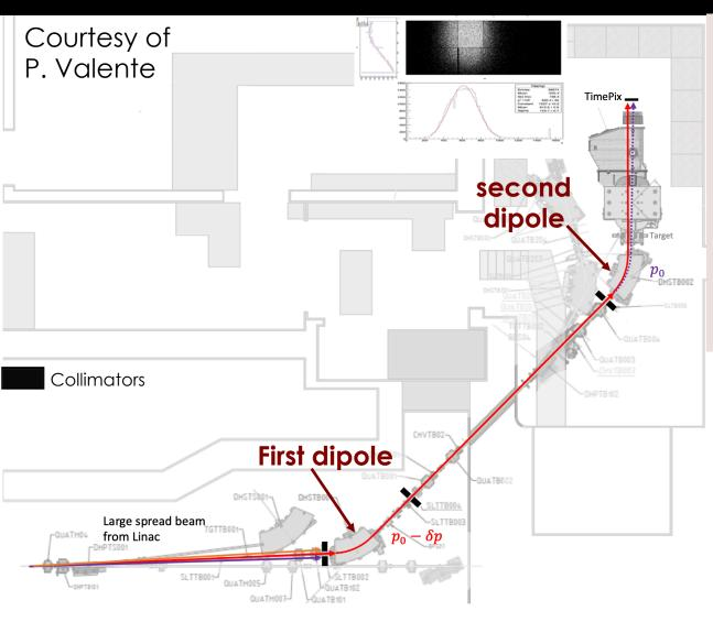
Use the first dipole magnet and collimators to select energy
