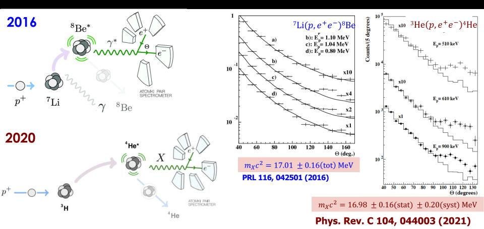
**ATOMKI** has confirmed the anomalous peak in the angular distribution of internal pair creation in <sup>8</sup>Be with a similar one in the <sup>4</sup>He transitions, with different kinematics but at the same invariant mass value.
