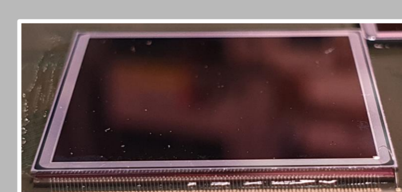
iLGAD bonded to JUNGFRAU 1.1 ASIC
