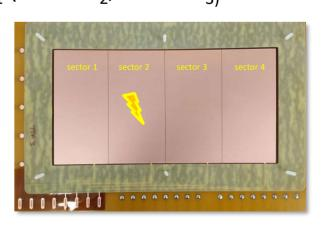
✓ The current flowing through the other sectors and foils is proved to be stable. No abnormal leakage current or discharges were detected during several hours of measurement
