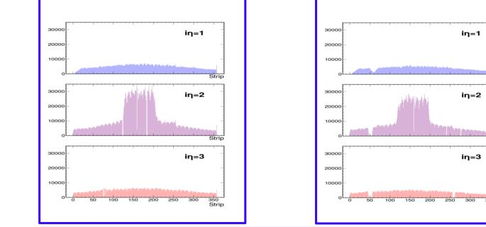
Strip profiles from CMS-ME0 modules assembled with blank (Left) and Random (right) segmented foils from June 2022 Test Beam
