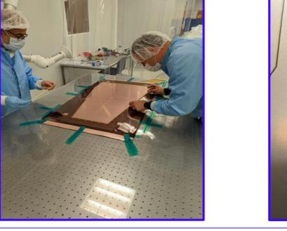
Large triple-GEM module (CMS-ME0 shape) assembled in March 2022 with "Random Segmented" foils Conclusion
