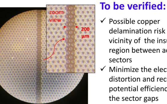
✓ Possible copper delamination risk in the vicinity of the insulating region between adjacent sectors Minimize the electric field distortion and recover the potential efficiency loss at the sector gaps
