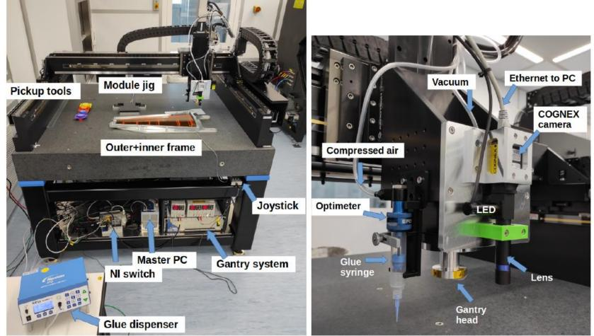
Automated pick & place and glue robot to mount modules to petals
