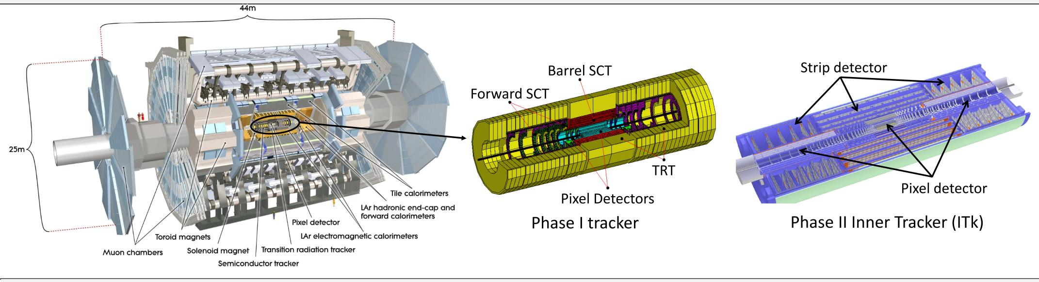
The High Luminosity Large Hadron Collider (HL-LHC) upgrade will require an upgrade of the ATLAS Inner Detector system. An integrated luminosity of 4000 fb<sup>-1</sup> and about 10 times higher track density compared to Phase I requires high granularity and high radiation tolerance of the Phase II tracker.
