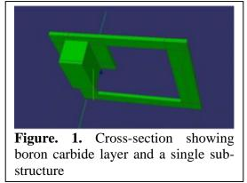
Using 3-D sensors allows for an increase in the thickness of the deposited  $B_xC$  layer, and thus an increase in conversion efficiency. However, the optimal coverage of boron does not necessarily correspond to the best detection geometry, nor what is manufacturable reliably.
