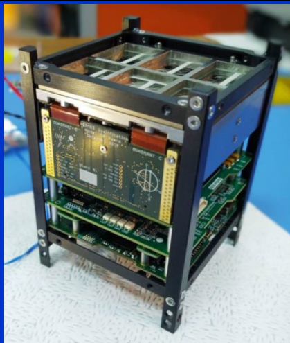
CubeSat 3U 10 \times 10 \times 30 \text{ cm}^3
