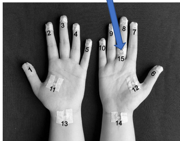
Fig. 4. Hand dose distribution of different TLD positions while working in a hot lab with ^{99m}\text{Tc} .
