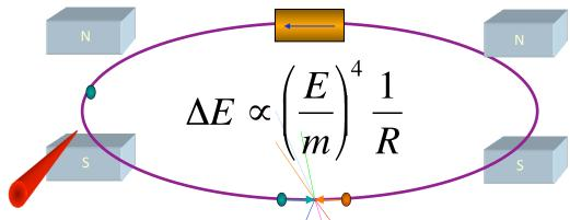
**Electron-positron linear colliders** avoid synchrotron radiation, but are **single pass**Typically cost proportional to energy and power proportional to luminosity, **RF limited**
