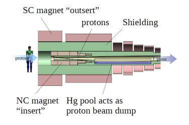
Hybrid design (superconducting + conventionnal magnets)
